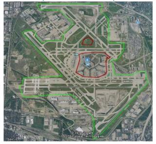
VTU-20 uses FAA approved Squitter Transmit Maps to automatically enable and disable transmission based on its location on the airfield.
