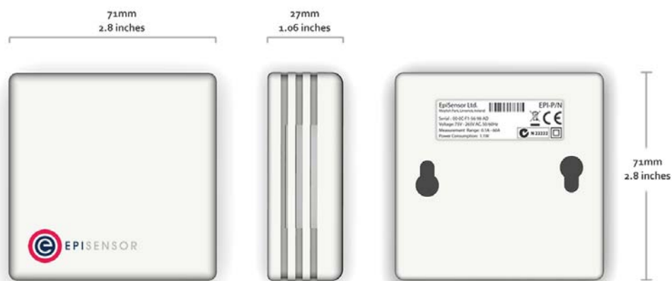
Dimensions for TES-11 / HTS-10 Wireless Temperature / Humidity Sensor
