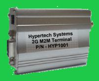
M2M Terminal is an easy to use plug & play 2G cellular modem with extended MMS capabilities. Based on Sagemcom's Hilo embedd modem, the 2G M2M Terminal is controlled by standard AT Commands via serial RS232 interface and standard DB9 connector, with its robust aluminum case, it enables the usage in harsh industrial and control environments.
