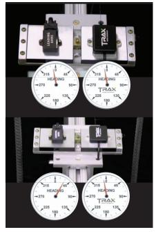
When exposed to magnetic distortion, TRAX maintains accurate heading — while the leading AHRS is thrown off track.
