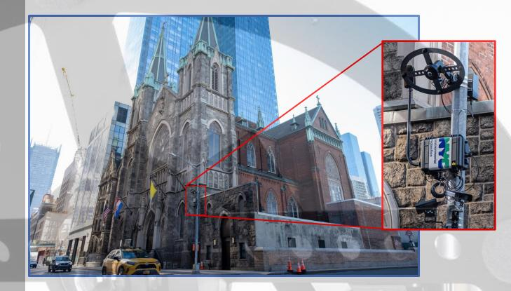
Following the New York City pilot refinements were made to the system which included provision of ANPR/ LPR cameras, a wide angle/ vehicle tracking camera and a microphone array which is used to detect the dominant noisy vehicle (even when there are multiple vehicles in the imagery).
