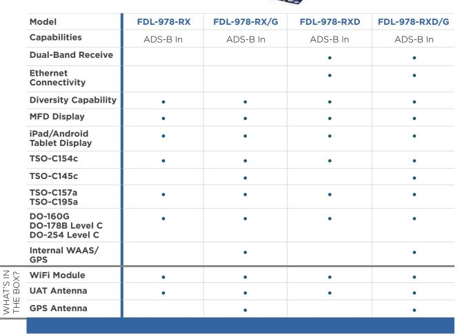
All RANGR systems weigh in at less than two pounds - weight includes antennas and coax cables. Units are TSO'd and STC approved in accordance with AC 20-165B and AC 20-172A.
