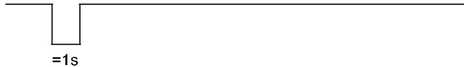
When an MG301 B2B Module receives a voice call, a periodical low level signal for 1s and a high level signal for 4s are output by RING, as shown in Figure 3-10 .
