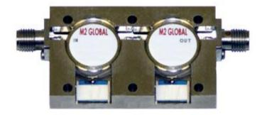
These modular design isolators and circulators provide coax units with the inherent advantages of drop-in devices, including good heat sinking, high power terminations, and 20/30 dB tabs for reverse power monitoring. Models H01, H02, and H03 can be equipped with terminations, up to 75W, while model H04 can have terminations up to 200W. The smaller H03 models can be used at frequencies up to 14 GHz. Optional mounting hole patterns are provided.
