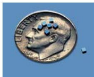
Micromachined Tilt Sensor Element
