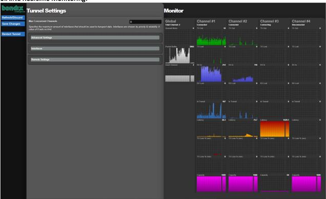
All status information can be queried via command-line interface, a custom API or SNMP and can be easily integrated in existing monitoring platforms like Nagios or comparable products.
